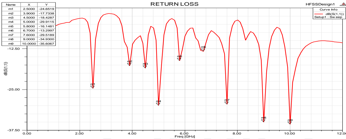
Fig: scattering parameters of rectangular patch antenna
