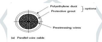
Strand cables are composed of parallel or helically combined strands:
