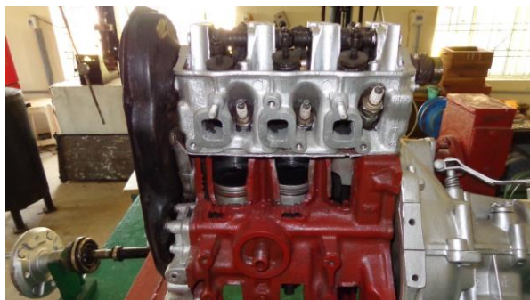
Fig. 1 Cut section of 3Cylinder 4 Stroke Petrol engine
