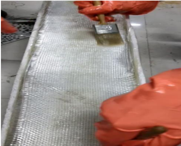
Fiber orientation of 90 and 0
