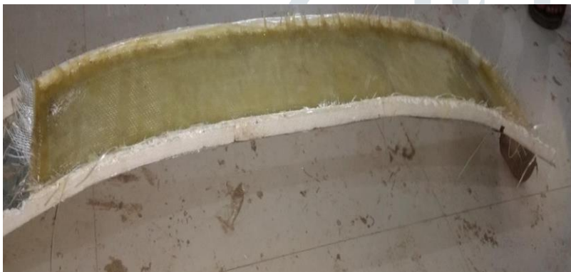
Curing of composite leaf spring
