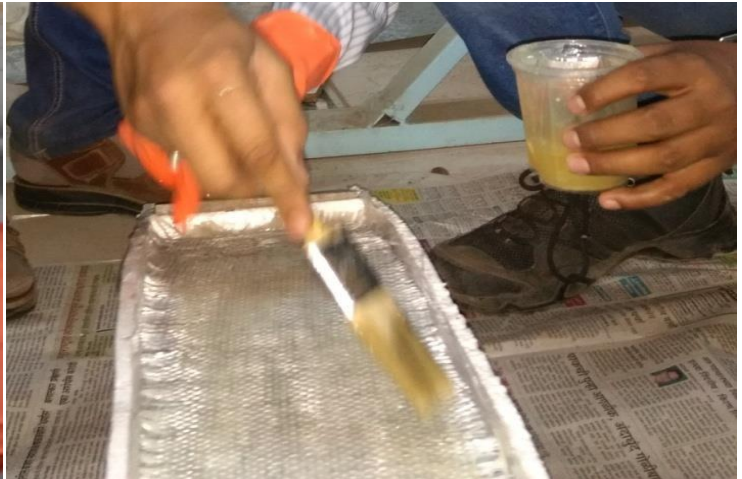
.Fiber orientation of 45 and -45
