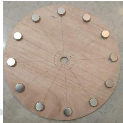
Fig 6. Placement of Magnet for stator
