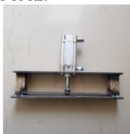
Fig.1: double acting cylinder
