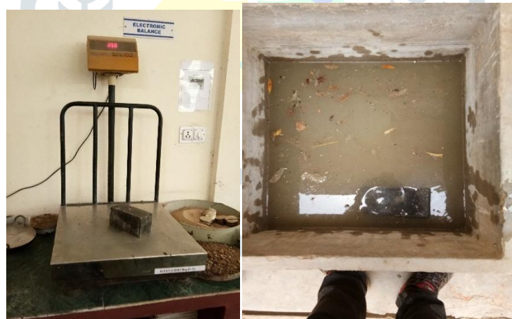
Fig 2 : Water absorption Test
