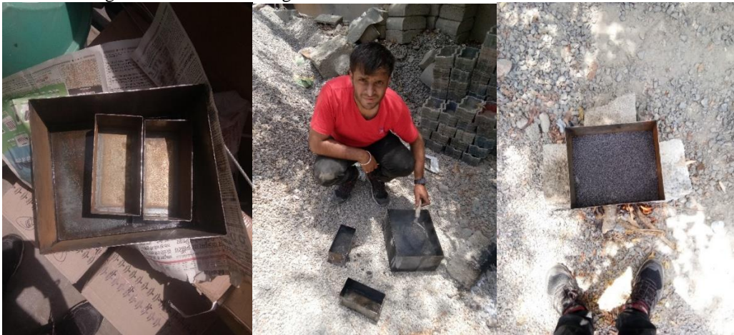
Fig 1: Making of Plastic Sand Bricks
