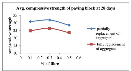
Fig No 3: Average Compressive strength of paving blocks at 28 days.
