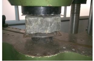
Fig No 6: cross sectional view loading test specimen for flexural strength
