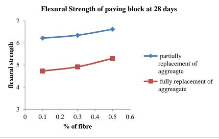
Fig No 9: Average Flexural Strength of paving blocks at 28 days.
