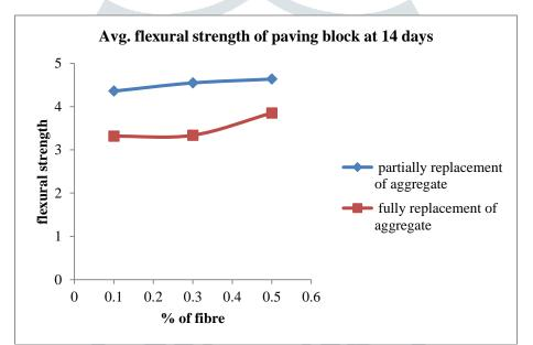
Fig No 8: Average Flexural Strength of paving blocks at 14 days.
