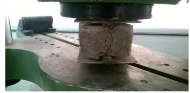
Fig No 10:Split tensile Strength Test Setup
