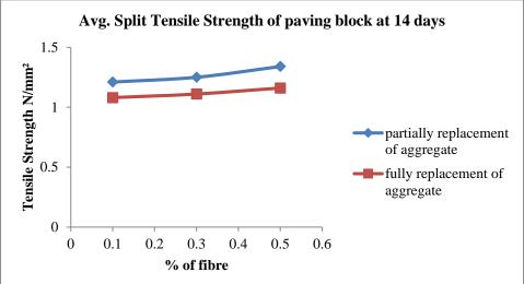
Fig No 11: Average Tensile Strength of paving blocks at 14 days.
