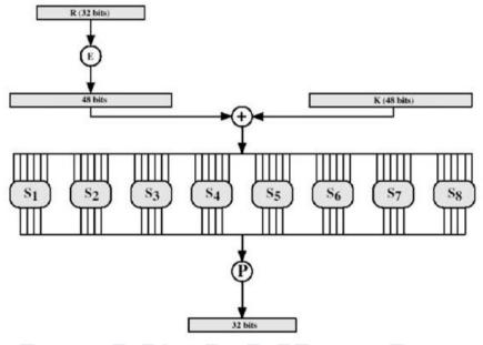
Fig 2.4: The Complex F Function Of the DES algorithm
