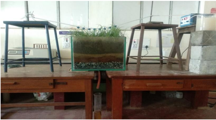
Fig 3: Experimental set for vermi biofiltration treatment
