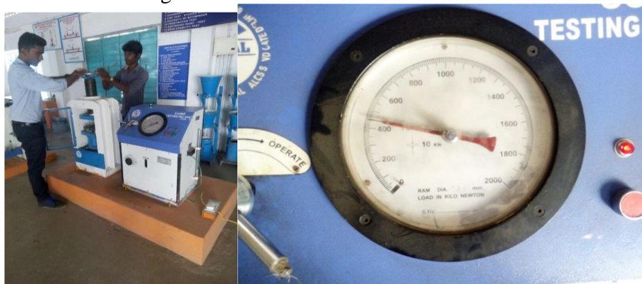
Fig 6.1 Compression test on blocks
