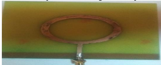
Fig.2 Ring line feed antenna implemented on FR4.
