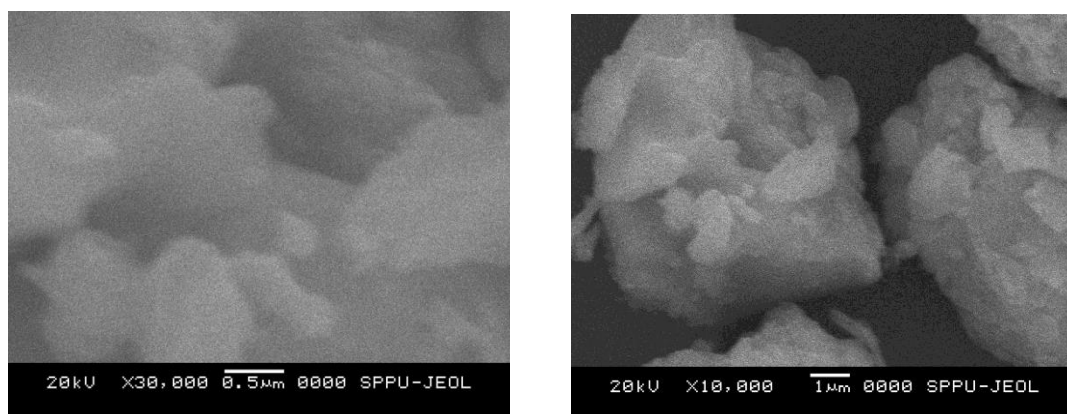
Figure 4: SEM image of CdS thin films deposited at 0.1 molar thiourea concentration
