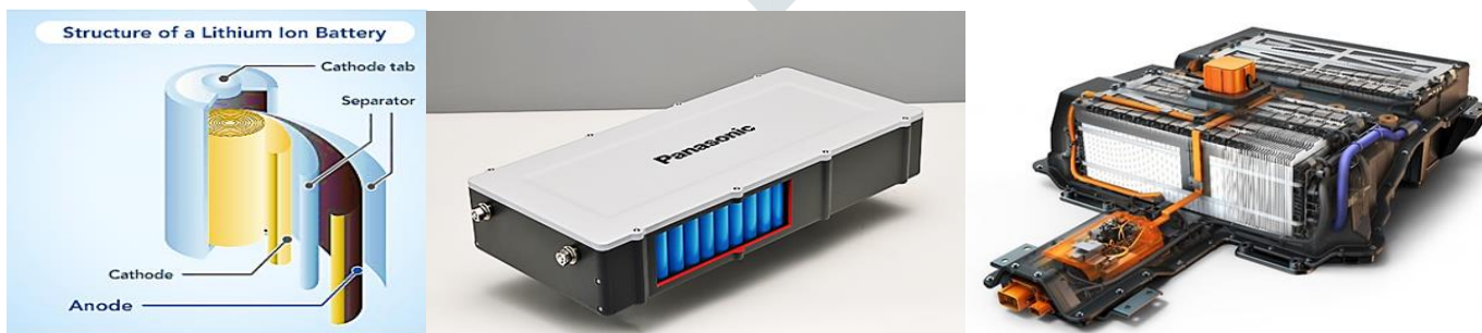
Fig.2: Li-ion Battery Cell, Battery module & Battery pack [9]
