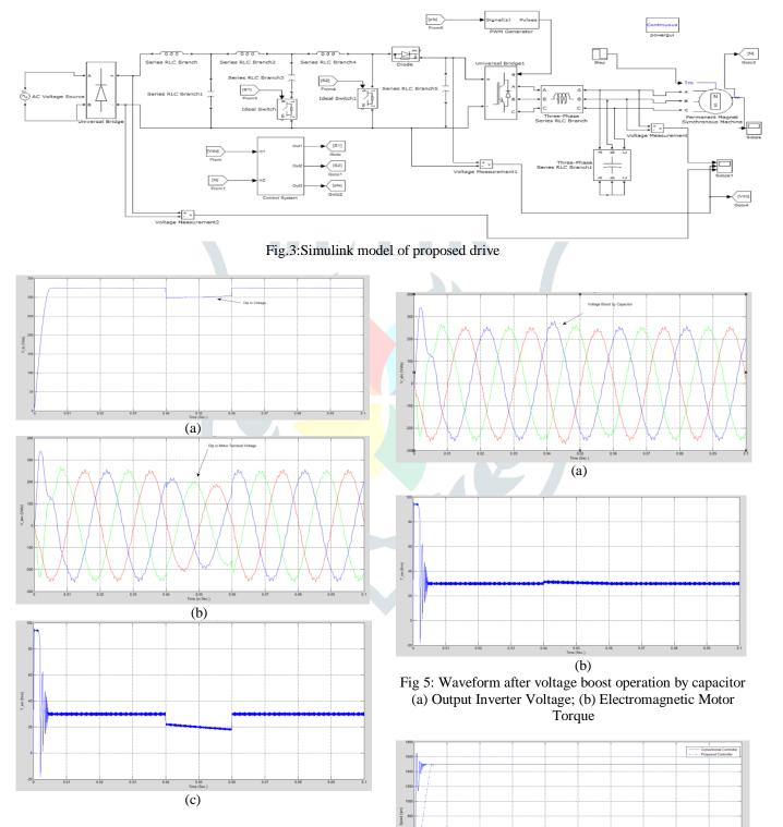
Fig 4:Waveform during low voltage disturbance (a) Rectifier DC bus voltage; (b) Inverter output voltage; (c) Electromagnetic motor torque
