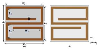
Fig. 2. The schematic diagram of NZIM unit cell: (a) Top surface[5], (b) Bottom surface[5]; ax = ay = 4.5 mm, L1 = 4.2 mm, L2 = 4.21.725 mm, L3 = 1.2 mm, W1 = 4.3 mm, W2 = 3.5 mm, W = 0.25 mm.
