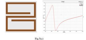
Fig. 5. design procedure of the proposed miniaturized NIM unit cell: (a) stage-1, (b) stage-2, (c) final proposed structure.
