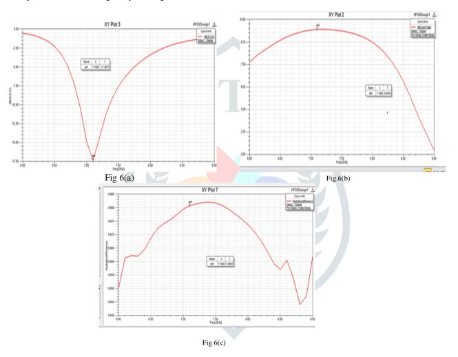
Fig.6 (a) Variation of simulated |S11| with frequency for proposed antenna with single layer NZIML. (b) Variation of simulated gain with frequency.(c) Efficiency of the patch antenna with NIZM unit cell.
