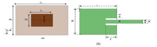
Fig. 1. schematic diagram of insect fed microstrip patch antenna: (a) Top view [5]. (b) Side view; Lp= 12.8635 mm, Wp= 17.3181 mm, Ls= 31.5 mm, Ws= 31.5 mm, S1= 3 mm, W1 = 1.4798 mm
