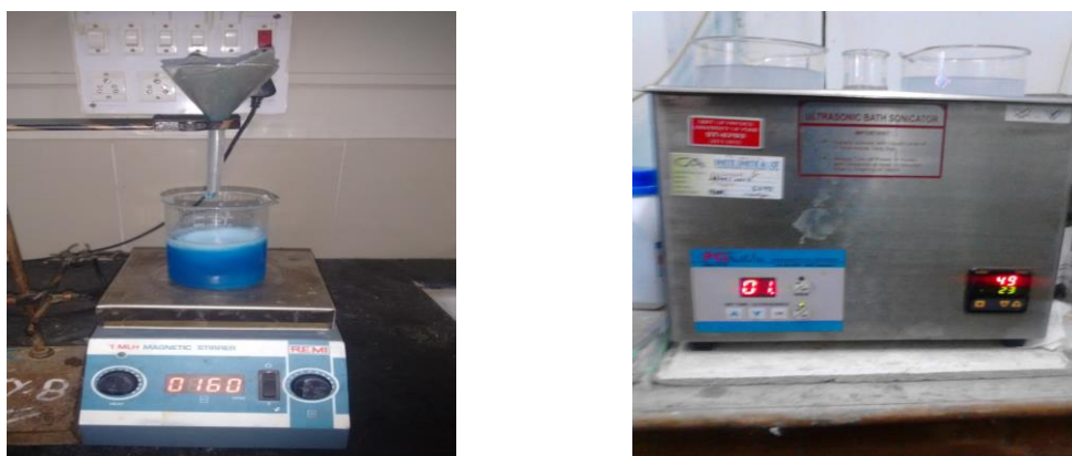
Figure 1.1: (a-b): Magnetic stirring and sonification of nanofluid
