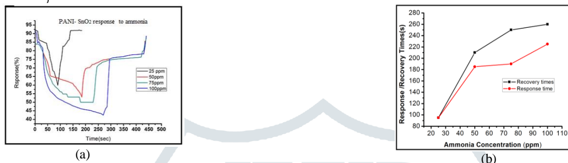
Fig 6. (a) Chronometric response of polyaniline–SnO 2 nanocomposite based chemiresistor to ammonia (b) Response-recovery times for different concentrations of ammonia.
