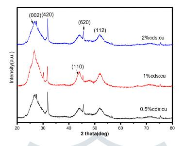
Figure 3.1- X-ray diffractograms of Cu doped CdS nanoparticles
