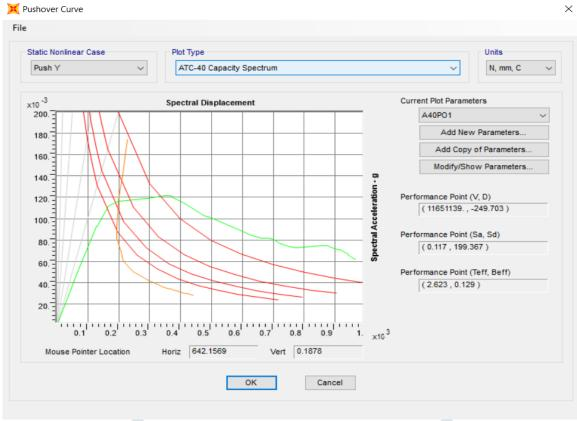
Figure 12 Capacity Curve for Push Y
