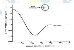
IS 11504 – 1987 gives the coefficient for circumferential variation of wind pressure in hyperbolic cooling towers. Asper the code (clause 5.1.3 and 6.2 - A- 2), the windpressure distribution on the outside of the shell is assumed to be symmetrical about the center line in the direction ofwind.
