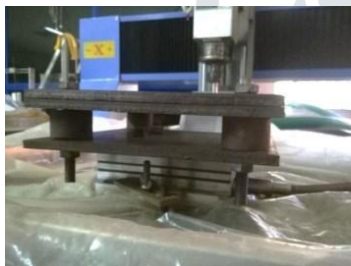
Fig. 3 Dynamometer clamped to the CNC table along with setup
