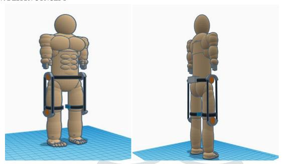
Our device consist of controller that generates signal which drives the motors and respective torque is generated by the motor which is transfer to thigh with the help of pulleys and belts assembly which move leg forward or backward. The proposed model will look like above figure.
