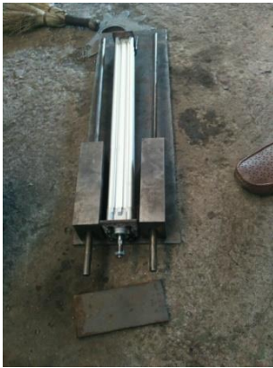
Fig 4. Fabricated Guide mechanism with actuator
