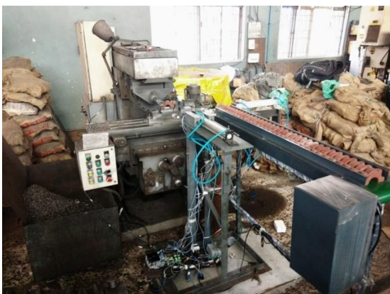
Fig 5. Automation setup for loading and unloading in SPM
