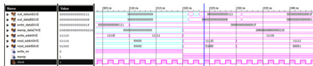
Fig. 10. Simulation result of the Hamming Code technique
