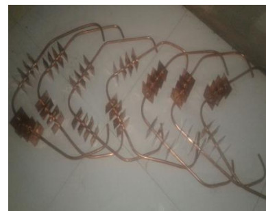
Fig.5. Braced copper tubes
