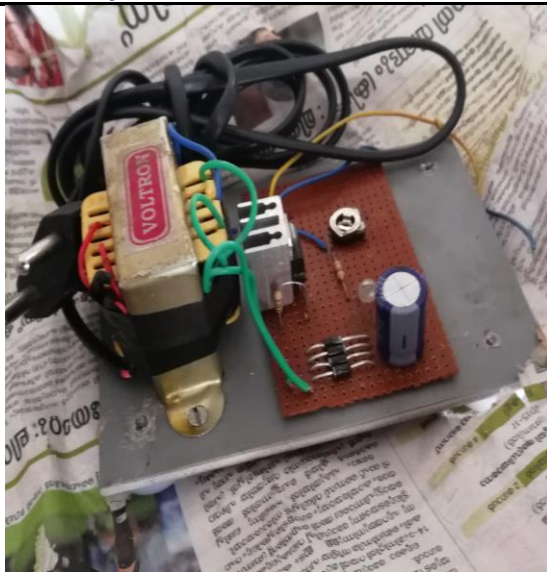
Fig. 4: Device used for supply of constant voltage of 16.5V
