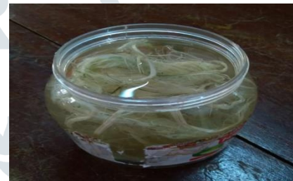
Fig.3 Water absorption test
