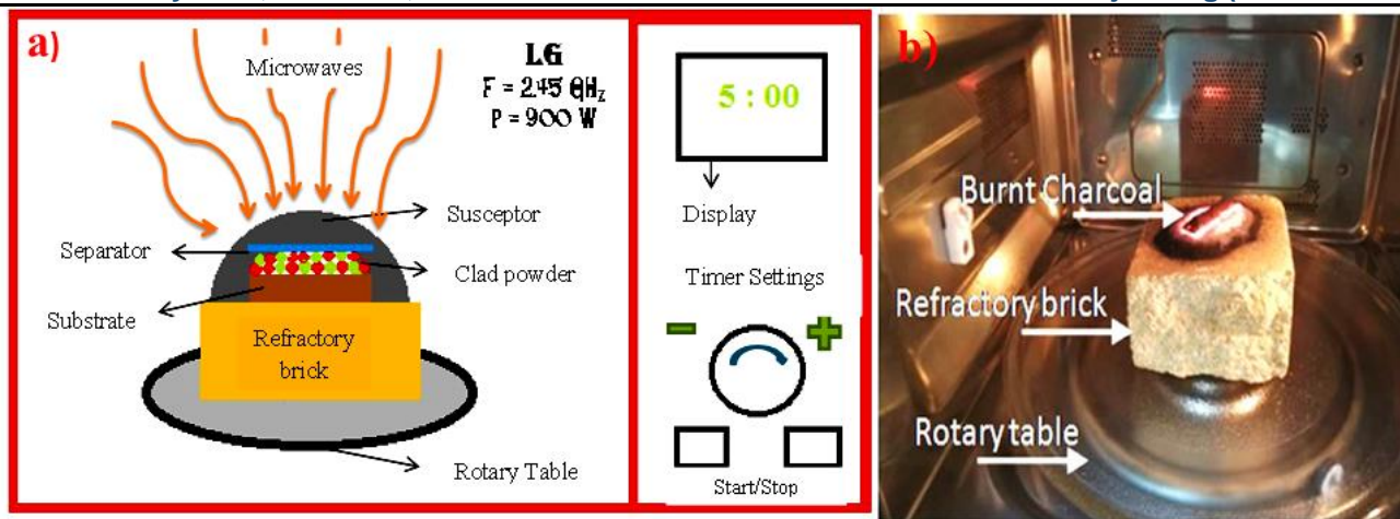
Figure 3: Clad deposition process through MHH (a) Schematic Principal (b) Actual Setup
