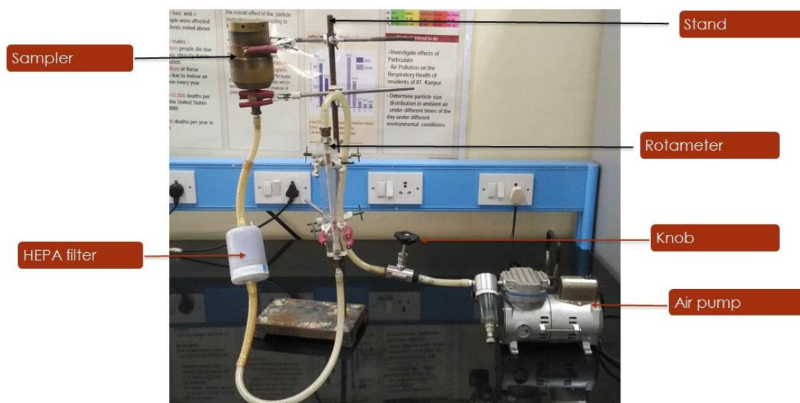
Fig. 1: Sampling setup of bioaerosols sampler (Chauhan, 2016).
