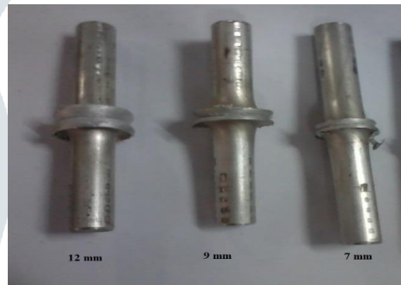
Fig. 2: Friction Welded Specimen depicts various burn-off lengths
