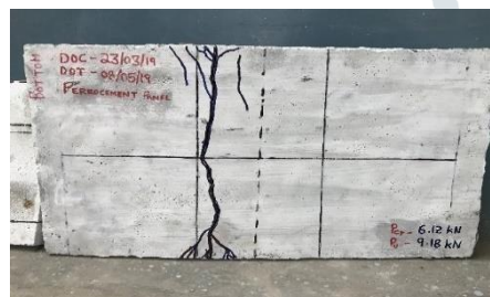
Fig 4 (a): Crack pattern of two point loading flexural test in longer span
