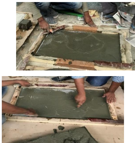
Fig 1 (b): Casting of panel specimens
