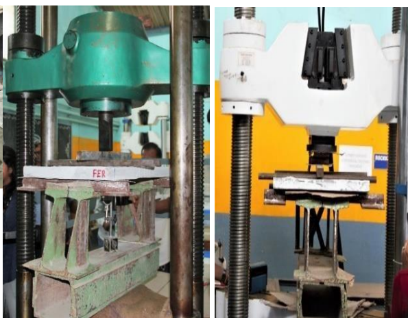
Fig 2: Flexural testing of panels
