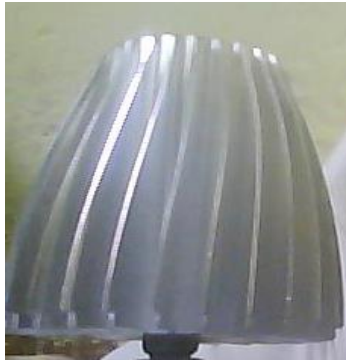
Fig 3 – Lotus type wind turbine curved aluminum blades
