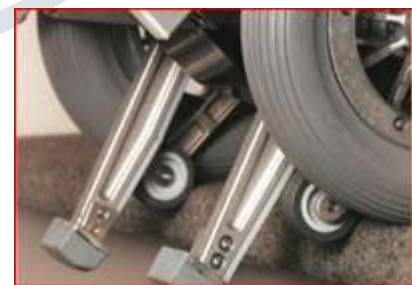
Fig 2.10 C-MAX U1 Climbing a Staircase
