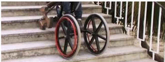
Fig 2.3 Vardaan Manual Stair-Climbing Wheel chair
