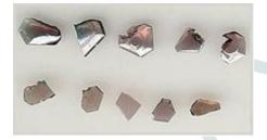
Fig 2. Synthetic SiC lely crystals
