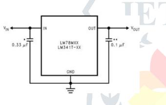
We have a 5V power supply circuit using LM 7805 IC. LM7805 is a famous positive voltage regulator IC, comes in three terminal provides fixed 5V DC output. This IC has many built in features like internal current limiting, thermal shut down, operating area protection etc. The IC will become hot during the operation so it is essential to use a good heat sink.
