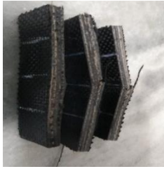
Fig. 23. Flexural test Specimen of Carbon Banana-Jute composite after testing
