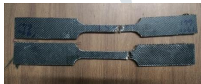
Fig. 15. Tensile Samples of Specimen B after testing
