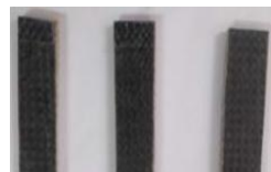
Fig. 21. Flexural test Specimen of Carbon Banana-Jute composite (Specimen B)
