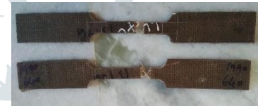
Fig. 11. Tensile Samples of Specimen A after testing
