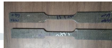
Fig. 10. Tensile Samples of Specimen A before testing
