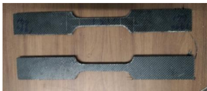
Fig. 14. Tensile Samples of Specimen B before testing
