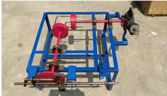
Fig-7: Gearless power transmission for skew shafts
