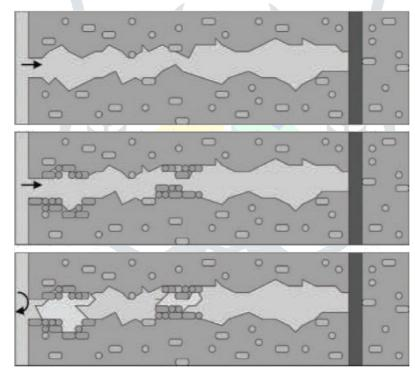
Figure: Scenario of crack-healing by concreteimmobilized bacteria (Jonkers 2007). Ingress water activates bacteria on fresh crack surfaces, bacteria start to multiply and precipitate calcium carbonate, which eventually seal and plug the crack and protect embedded steel reinforcement from further external attack.
