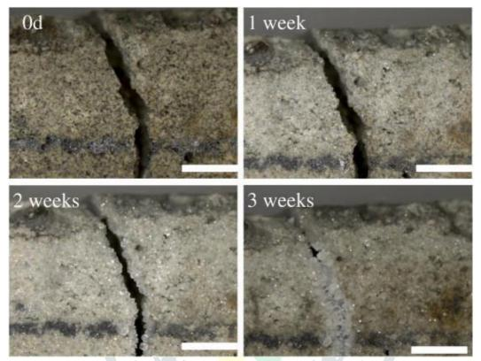
Figure: this shows how the crack is healed over the period of time.
