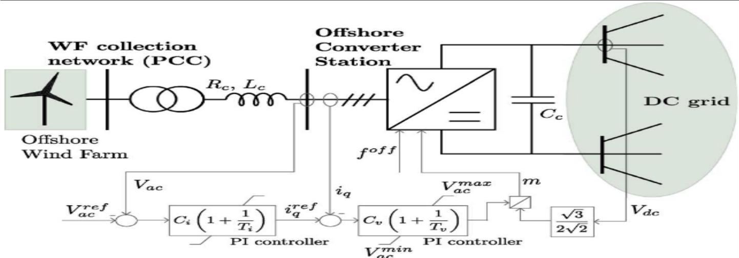
Fig1. 2: Control of Offshore converter
