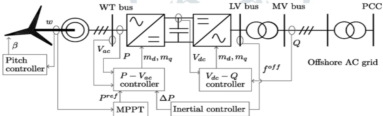
Fig 2.1: Wind turbine generator control
