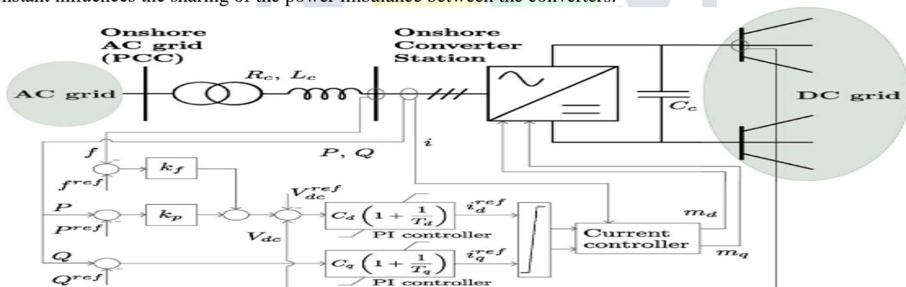
Fig 1.1: Control of Onshore converter
