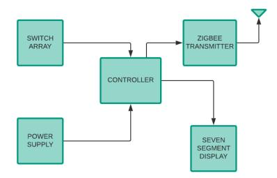
In the above figure-1.2 it consists of a microcontroller, a zigbee transmitter and a seven segment display. At this node, transmission of message signals via a zigbee transmitter takes place to the master control unit. These message signals are further received by the master control unit with the help of a zigbee transceiver.
