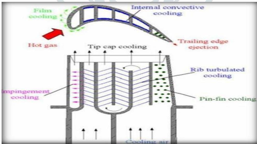
Fig.2 Internal convective cooling [5]
