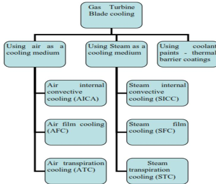
Fig.1 Classification of the blade cooling
