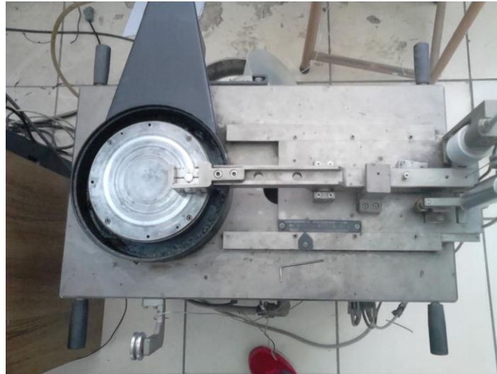
Figure 11. shows Pin on Disc setup
