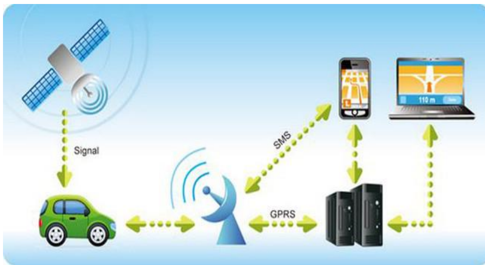
Figure 1. Working of Global Positioning System.
