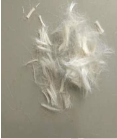
Fig.1 - Recron 3S fiber packets manufactured by Reliance Industries Ltd.
