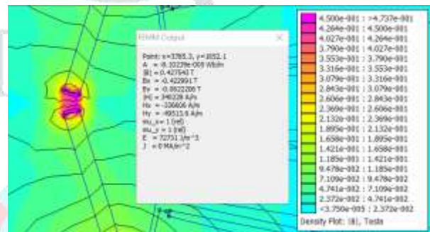
Fig 10: The result of the flux density plot
