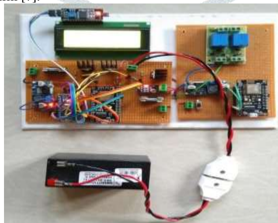
Figure 3.1: Biogas consumption details through Wi-Fi module
