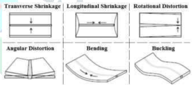
Fig-1: Types of weld distortion
