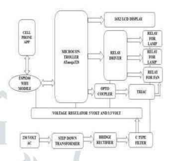
Fig-1: Block Diagram of IoT based Home Automation
