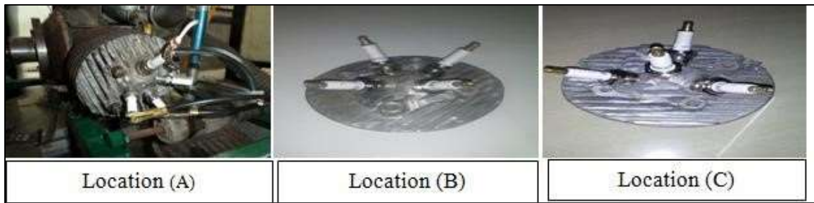
Fig. 1: Location Four Spark Plug on Cylinder Head
